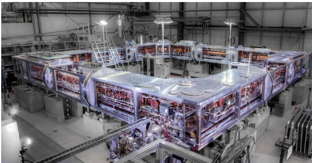
Figure 4: The Heidelberg CSR is the largest electrostatic storage ring project in the world. It has a circumference of 35.1m and a nested cryogenic vacuum structure. The electrostatic deflection makes it a very versatile instrument for molecular physics, as it does not impose any mass limit on singly charged ions (in stark contrast to magnetic storage rings). In the first commissioning phase in 2015, the inner experimental vacuum chambers reached a pressure better than 10^{-14} mbar and temperatures of 5 K.
